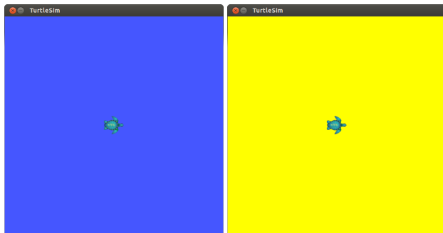
Figure 7.1: Before (left) and after (right) a change to the background color of a turtlesim node.
